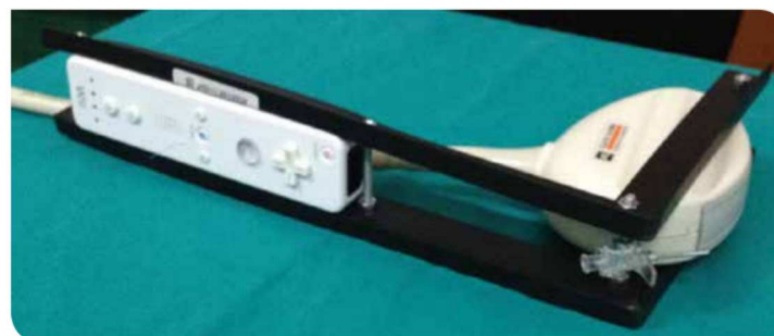
Fig. 2: The Wiimote and the biopsy kit, rigidly attached to the ultrasound probe
