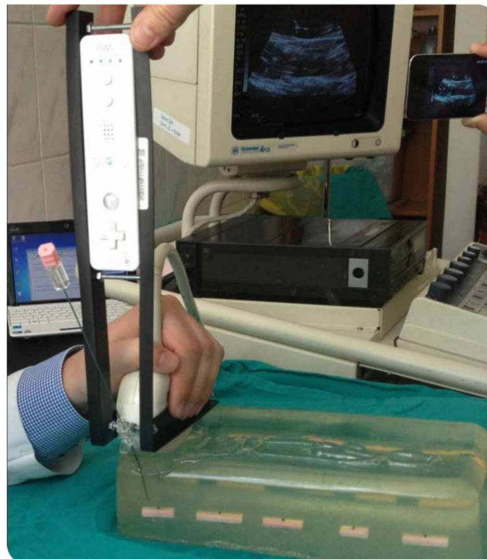
Fig. 3: The in vitro experiment using the ultrasound probe with the Wiimote and the puncturing system on the marked silicon tubes immersed in the ballistic gel
