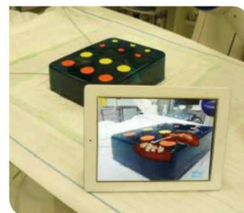
Fig. 3: Projection of the kidney on the ballistic model with the iPad
